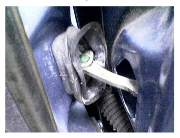
These are quite difficult to get at because the door is in the way so you can't just get something straight on. I used a short insert with a 10 mm spanner to turn it
