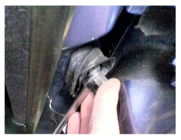
Then you can open the door just a bit wider, and get at the 2 x 10 mm nuts holding the whole Check Strap to the door. You will need a short 10mm sockets to get to these. Be carefull DON'T Drop the nuts into the door frame - it's easy to do, and you'll never find them again
