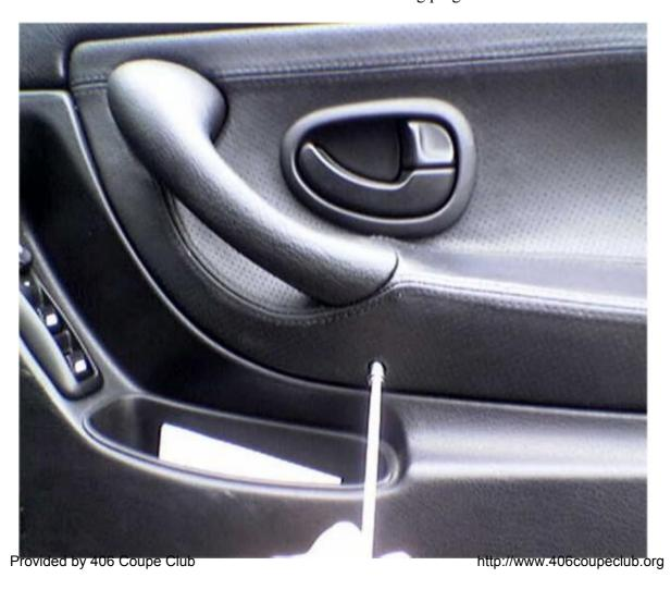
Then unclip the door opener with a flat screwdriver
